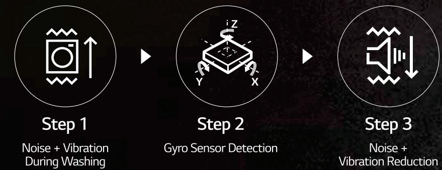
LG's Gyro Balancing Sensor precisely detects the tub movement to activate the most proper algorithm for washing cycle, ensure it finish within 36 mins.
